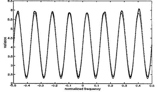
Figure 1. Variance of the HAF vs. frequency ( $M = 3$ ,  $SNR = 18$  dB) - theoretical results (solid line), simulations (dotted line).
