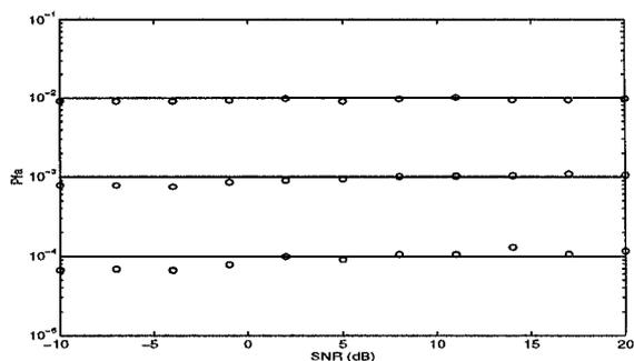
Figure 5. Estimated  $P_{fa}$ : desired values (solid line) and simulation results (circles).
